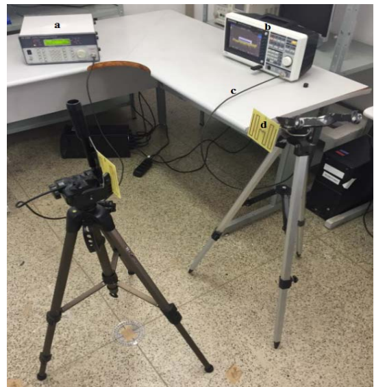
Fig. 6. Measurement setup of antenna radiation diagram: a) signal generator, (b) spectrum analyzer, (c) connector cable, (d) short dipole antenna.
