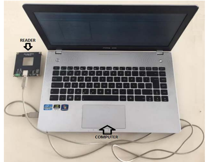
Fig. 9. Setup of measurements for the verification of the influence of temperature and aluminum on the performance of passive UHF RFID tags.
